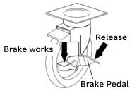
Right side flexible wheels have brake to lock wheel ① To lock - Push down of Brake Pedal in the front ② To release - Push down the Pedal in the back
